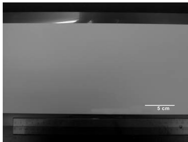
Fig. 1. Photograph of a LSGM sheet prepared by tape casting method.
